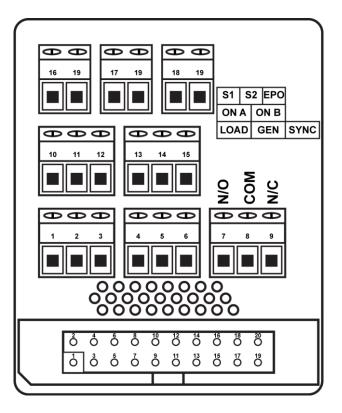
The relays can switch up to 50VAC/DC - 2A and are not suitable for 110/240V or other applied voltages Remote contacts are wet contacts and do not require external voltage to be applied.
