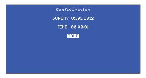
Entering the date and time should only be required once. We strongly encourage setting the correct time and date so that accurate real time event correlation can be undertaken. The real time clock is thereafter backed up by a battery cell.
