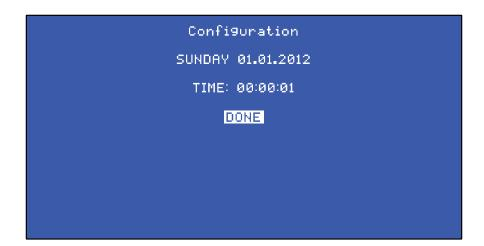
Entering the date and time should only be required once. We strongly encourage setting the correct time and date so that accurate real time event correlation can be undertaken. The real time clock is thereafter backed up by a battery cell.
