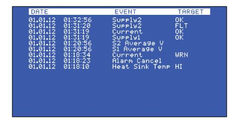
The Events List shows 200 logged events that are recorded in real time. Once the buffer is full, the oldest events will fall from the buffer and get replaced by any new events. Refer to Event Codes section under Fault Diagnosis for an explanation of the codes.
