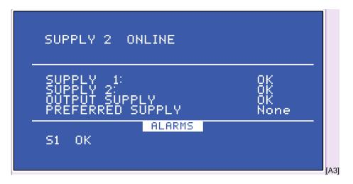
The Status & Alarms Screen shows the status of the STS status and the most recent fault alarm.
