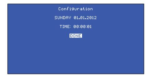
Entering the date and time should only be required once. We strongly encourage setting the correct time and date so that accurate real time event correlation can be undertaken. The real time clock is thereafter backed up by a battery cell.
